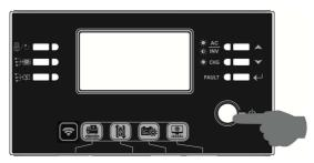
Step 4. Be sure to select battery type as "WEC" in LCD program 5.
